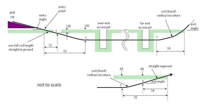
Figure 11 Drill Rig Setup and Related Distances (Source: Outside Plant Consulting Services, Inc.)
