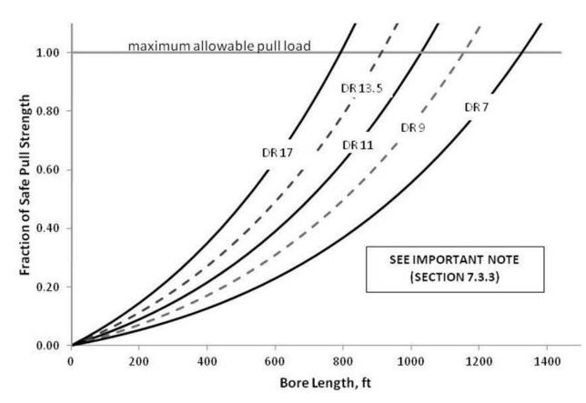
Figure 9 Predicted Mini-HDD Pull Load vs. Safe Pull Tension, HDPE (PE4710) Pipe Nominally Straight Path, 2-inch Drill Rods (Source: Outside Plant Consulting Services, Inc.)
