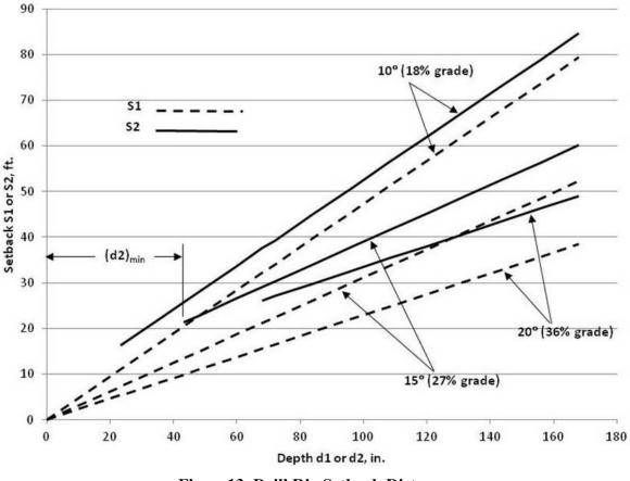
Figure13 Drill Rig Setback Distance Drill Rods: 6 ft Long, 60 ft Radius of Curvature (Source: Outside Plant Consulting Services, Inc.)
