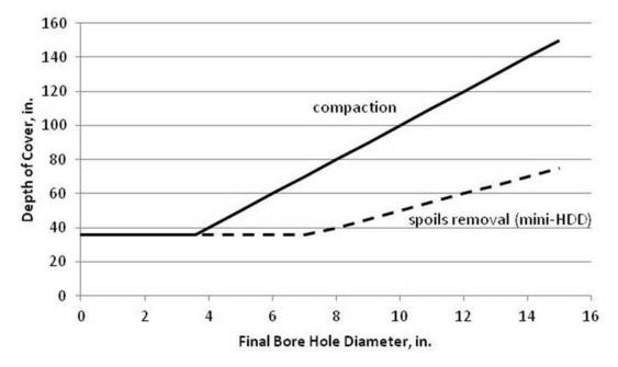
Figure 10 Recommended Minimum Depth of Cover (Source: Outside Plant Consulting Services, Inc.)
