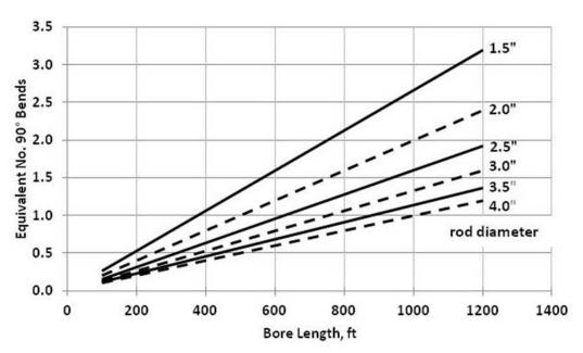
**Figure 8 Unplanned Curvature, n**<sub>2</sub> (Source: Outside Plant Consulting Services, Inc.)
