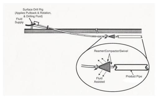
Figure 2 Typical Mini-HDD Back-Reaming and Pipe Pullback Process (Source: Outside Plant Consulting Services, Inc.)
