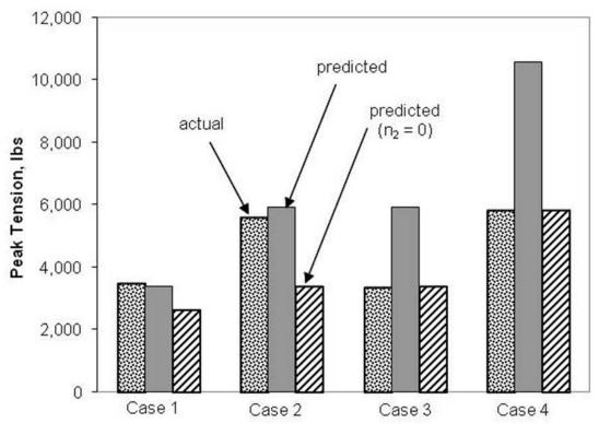
Figure D.1 Actual vs. Predicted Tension for Mini-HDD Installations
