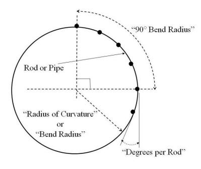
**Figure 3 Rod or Pipe Curvature Terminology** (Source: Outside Plant Consulting Services, Inc.)
